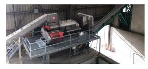
SMICON depackaging machines flawlessly separate metallic and plastic food packaging from organic material. Inputs can be grocery store or commercial food waste. The depackager decouples the packaging while screening the organics to create a pumpable organic stream. The packaging emerges as a relatively clean, dry material that can be sold to recycling or fuel markets. The organics are ideal inputs for composting or digester operations.
