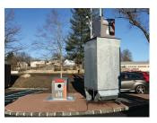
These sleek containers store waste and recyclables in underground receptacles. Storage capacity is vastly improved (33 times the storage of a typical 40-gallon waste bin), and the unit can be
