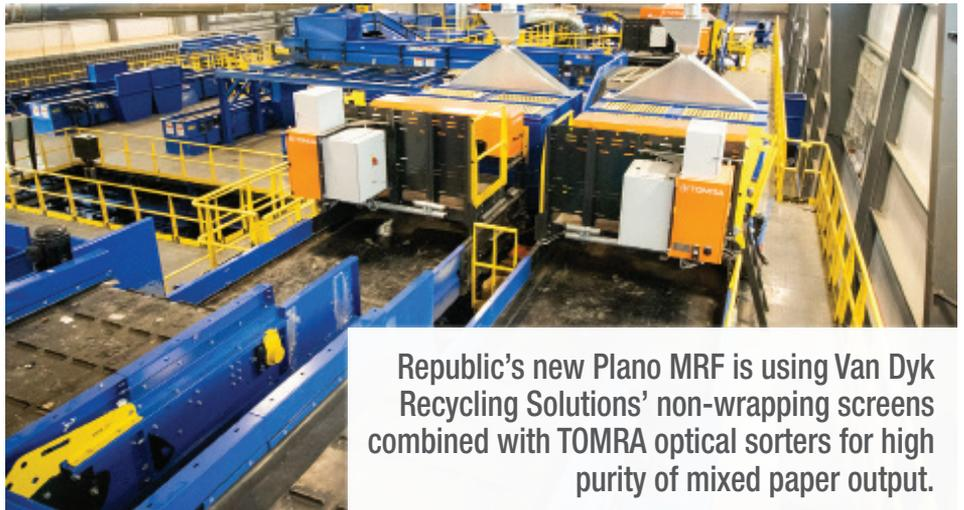
Republic's new Plano MRF is using Van Dyk Recycling Solutions' non-wrapping screens combined with TOMRA optical sorters for high purity of mixed paper output.
