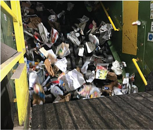
Screens are an integral component for separating a wide range of paper, plastics and other materials with maximum efficiency at MRFs and smaller recycling facilities. Cleaning these screens can be a challenge.
